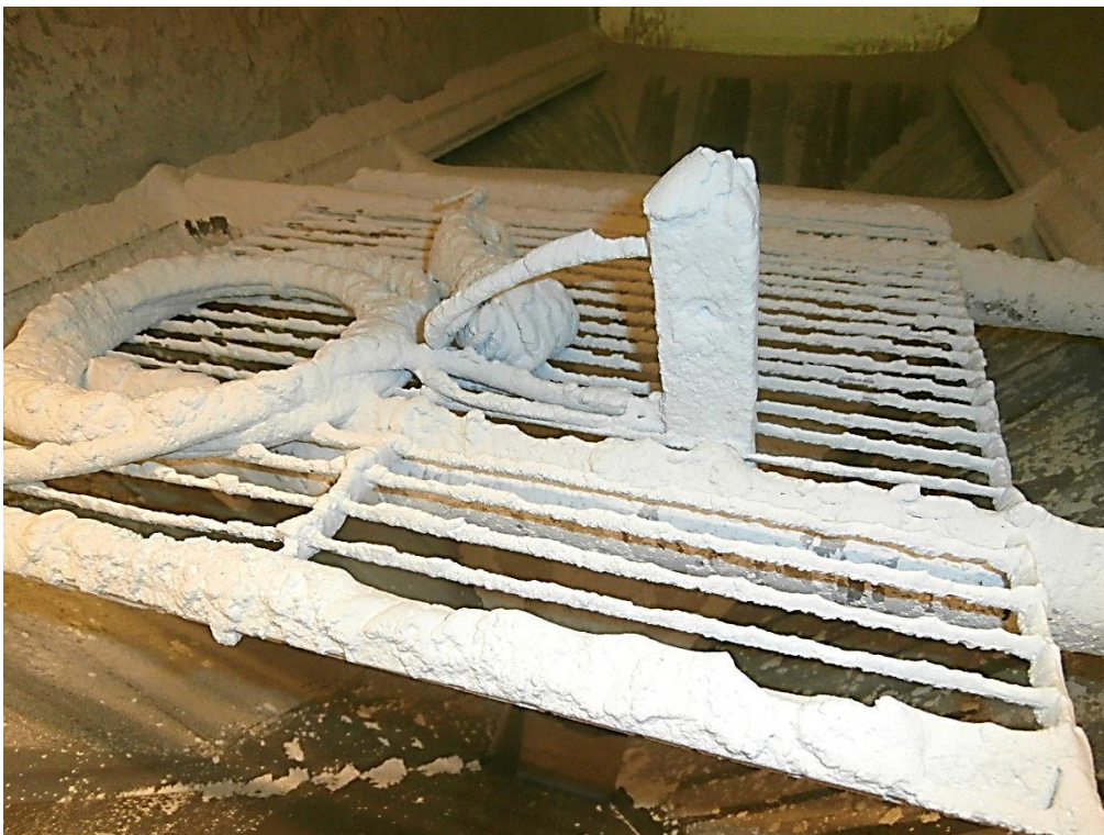
Photograph N°2: Equipment after test for the protection against ingress of dust (IP5X).
