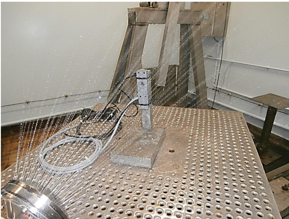
Photograph N°4: Equipment during test for the protection against penetration of water (IPX4).
