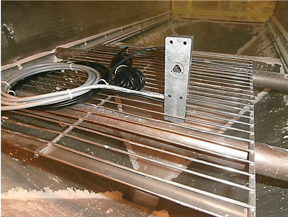
Photograph N°1: Equipment before test for the protection against ingress of dust (IP5X).
